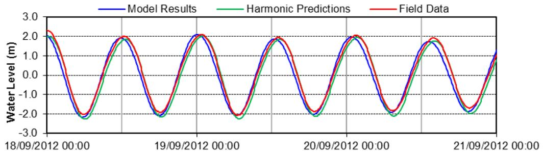
Figure A-5 Model calibration performance against water level: JN1163 North
