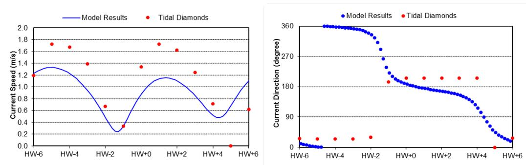
Figure A-33 Model fit during calibration period: SN062B
