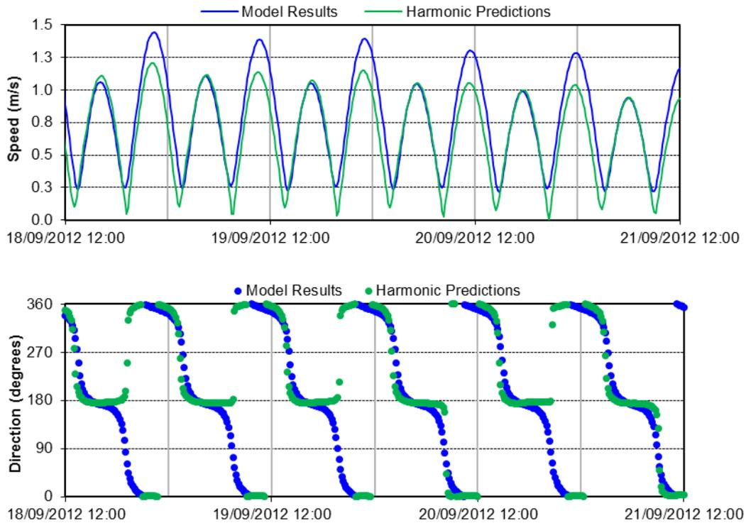
Figure A-23 Model calibration against current data: JN1163 North
