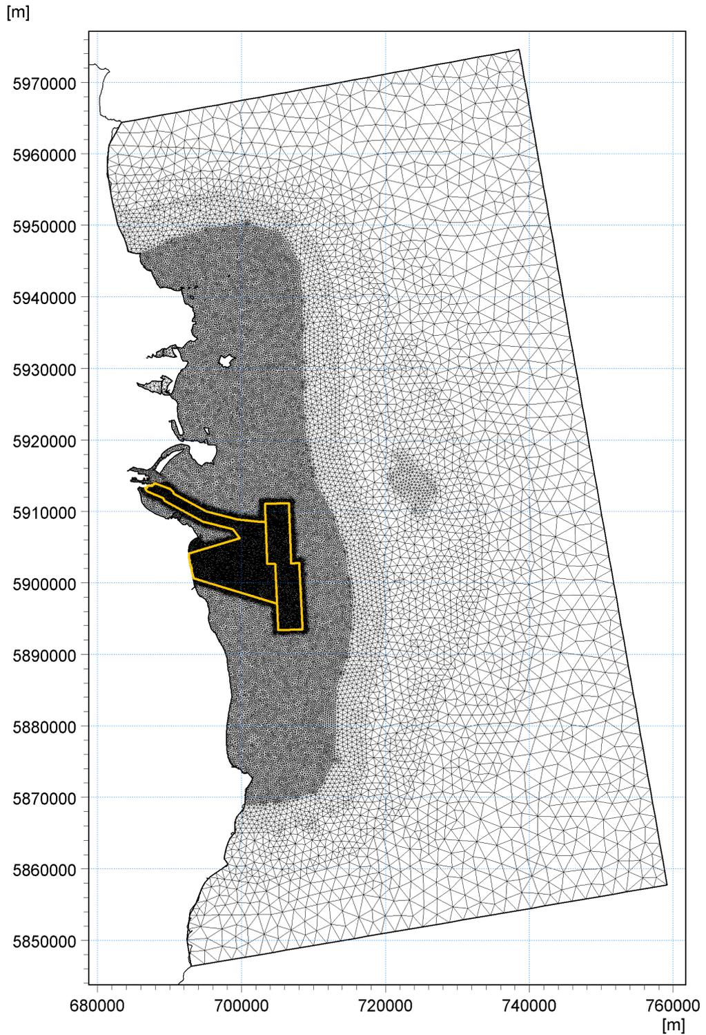
Figure 3-2 Hydrodynamic Model Domain and Mesh – proposed wind turbine area
