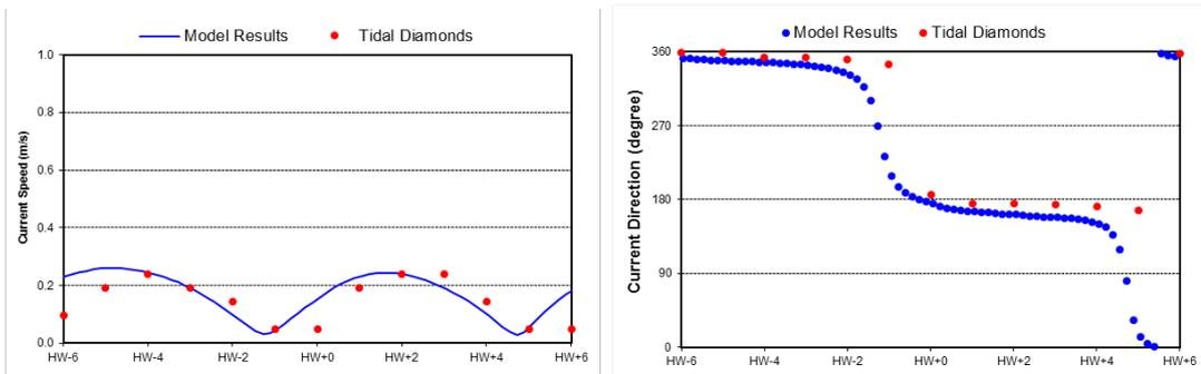
Figure A-42 Model fit during validation period: SN062D
