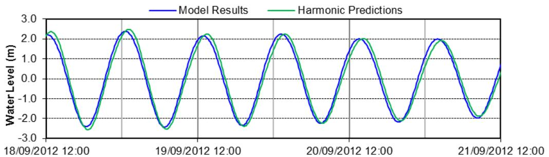
Figure A-10 Model calibration performance against water level: Wicklow
