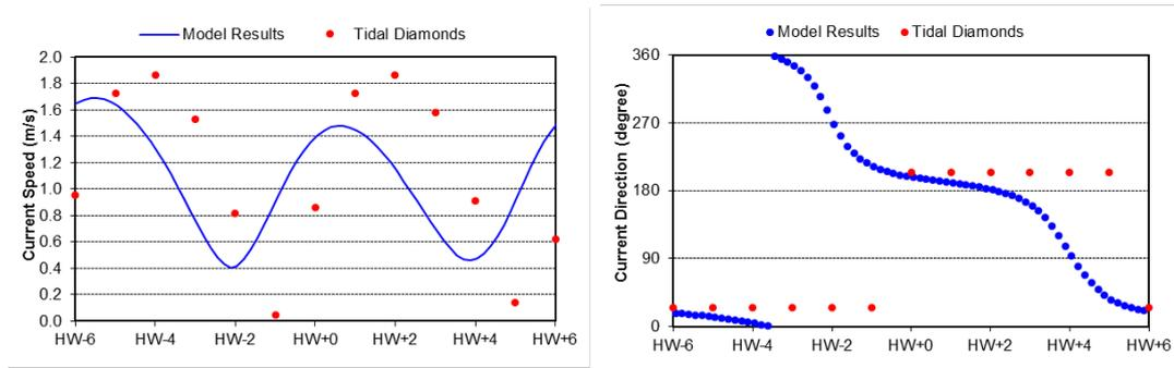
Figure A-32 Model fit during calibration period: SN062A
