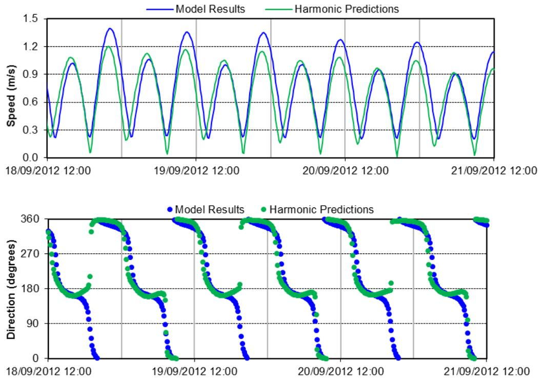
Figure A-22 Model calibration against current data: B014738
